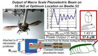
Figure 1: Setup used to find optimum location for energy scavenging, and measurement of available power during beetle's tethered flight.
